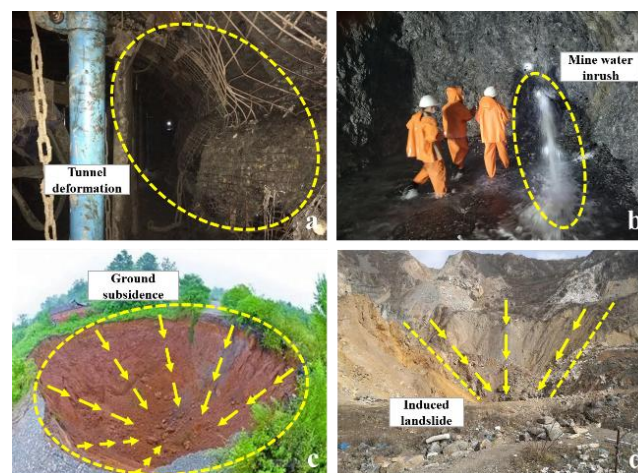
Fig. 2. Geological disasters and underground incidents stemming from overburden deformation
